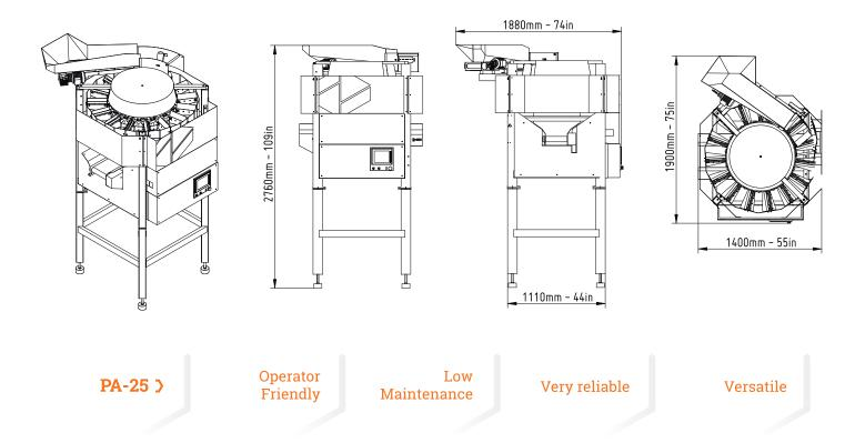
The PA-25 sets all weighing parameters automatically, achieving the best performance under any condition. Optional manual settings are available if a manual override is necessary.
