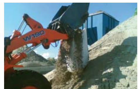
With a special tool the EXIM FIBC can be filled quickly.
