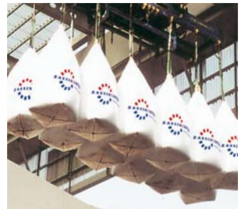
Zakkencentrale supplies practical equipment to hoist up to 12 FIBCs in one go.
