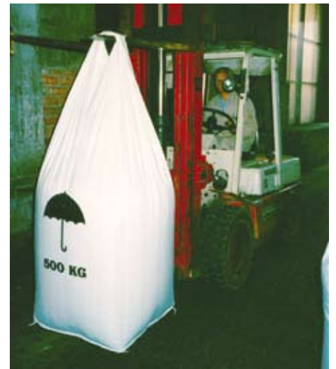
Two FIBCs can be moved using the standard forks of a forklift truck.
