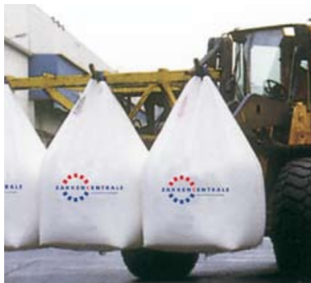
Appropriate forklift/spreaders are available to move several FIBCs in one go.
